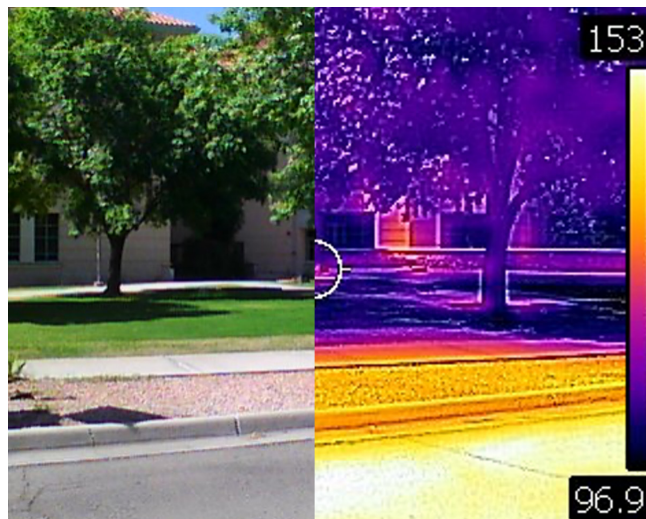
Figure 2.15. Thermal image (right) taken in Las Cruces, New Mexico, showing hotter areas in brighter colors with cooler areas in darker colors, with temperatures displayed in Fahrenheit (Dave DuBois/U.S. NOAA)
