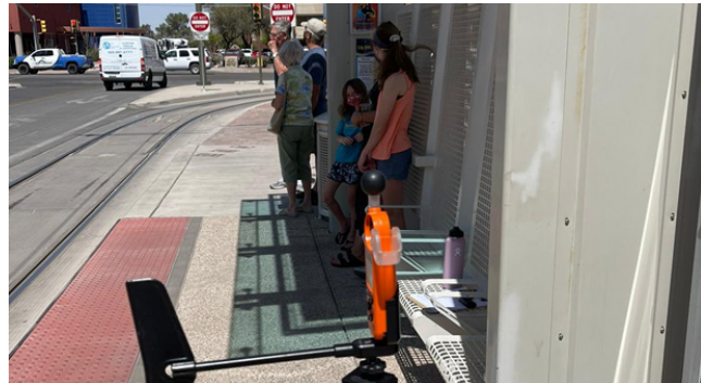
Figure 2.7. A portable device collects wet bulb globe temperature while Tucson Sun Link Streetcar riders find respite from the heat in the shade (Ida Sami, University of Arizona)
