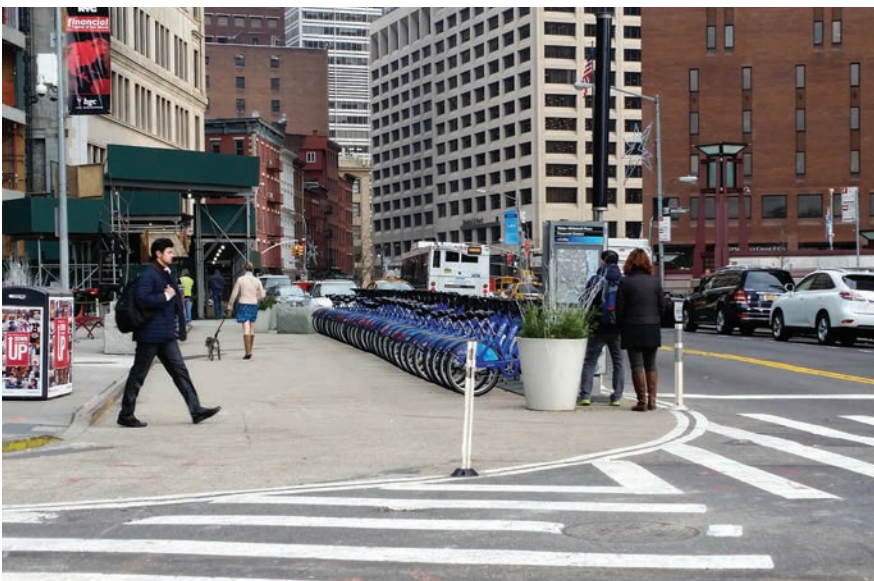
A bike share station forms a clear border for a painted curb extension on a busy street. Citi Bike. New York, NY
