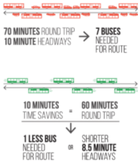
Example of operational savings from transit improvements.
